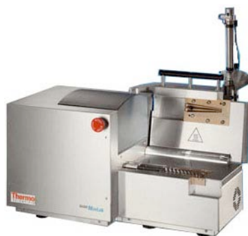
Figure 2.3 Haake minilab extruder from ThermoScientific at the Institute of Polymer Science and Technology (ICTP-CSIC, Madrid)
