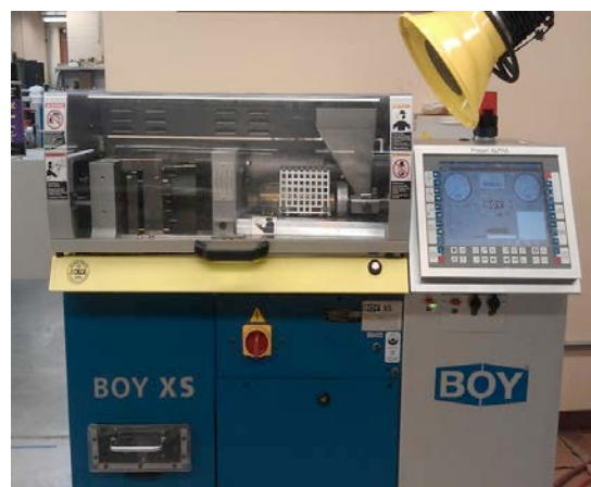
Figure 2.4 Boy XS injection moulding machine at the Polymer Engineering Center, University of Wisconsin – Madison
