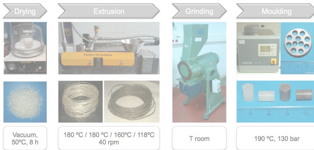
Figure 6.1 Process for manufacturing PLLAXMg and PLDAXMg composites
