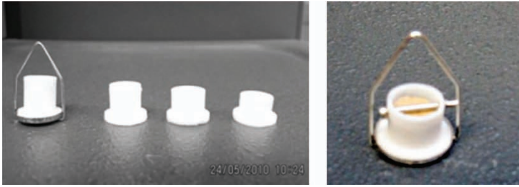
Figure 1. Teflon pans filled with Kraft paper or pressboard to the required thickness for thermogravimetric analyzer experiments.
