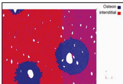
Fig. 4 – Meshed workpiece reproducing microstructure of bone (Hage and Hamade, 2013).
