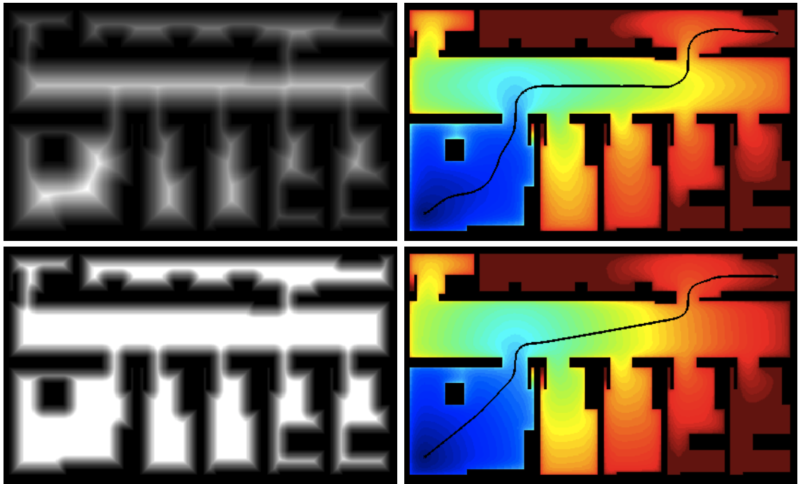
Figure 2.23: Motion trajectories obtained by the FM^2 . Example of FM^2 with both stages: the generation of the velocities map (left) and the calculation of the path (right). The velocity potential map is saturated on the bottom example.
