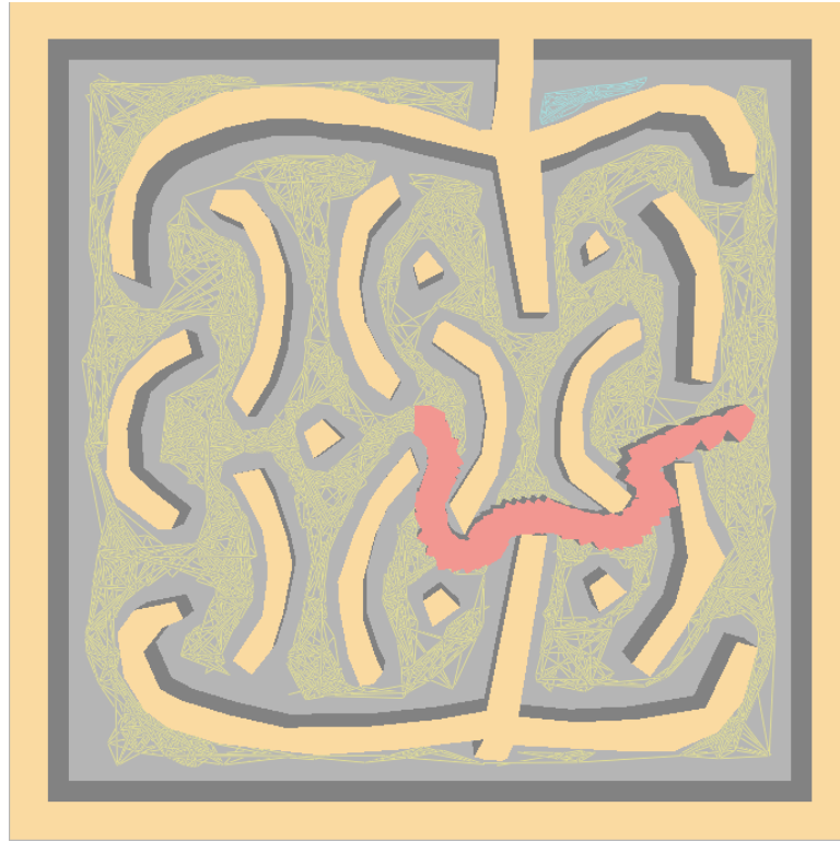
Figure 2.14: Example of an PRM search and generated path.
