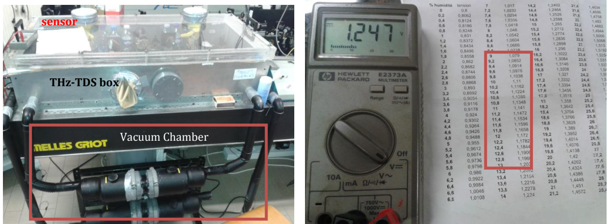
Figure 4.5: [Left] the THz-TDS set up in vacuum chamber. [Right] The sensor voltage to control relative humidity % in the set up (it has been optimized in 9~13 % corresponding 1~2 V).
