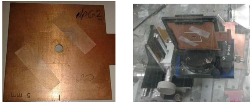
Figure 4.3: [Left] the sample holder with whole of 5 mm. [Right] the sample holder aligning and setting up in THz-TDS set up.
