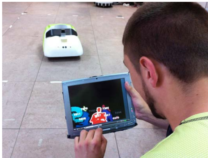
Figure 7.19: A sample picture of a user selecting the object-of-interest. It is indicated by the shape with a white border. The other objects are drawn with a different color.
