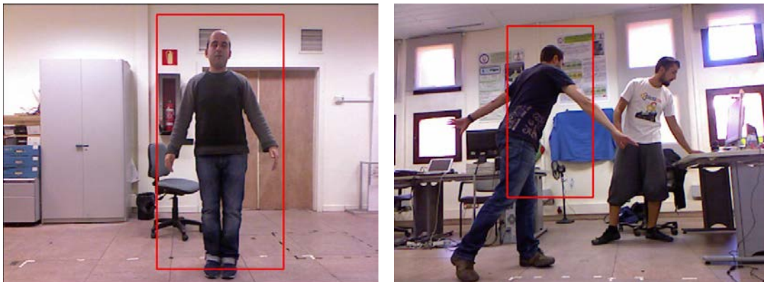
Figure 3.2: Sample detections with the original HOG algorithm. Note the miss detection on the right: the white user was not detected.
