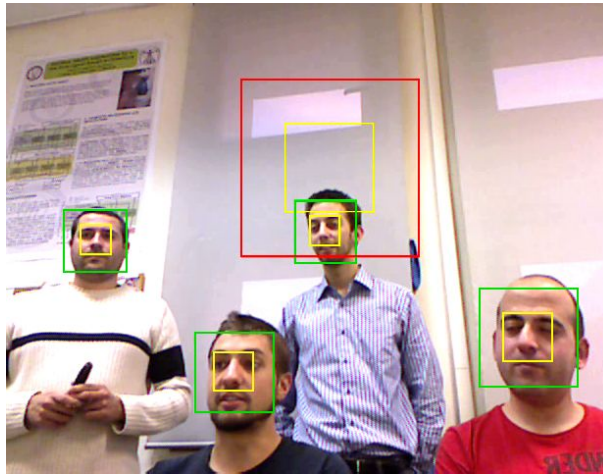
Figure 3.8: Results of the face detection algorithm on a sample image. The red and green rectangles correspond to the faces as detected by the Viola-Jones detector. The inner yellow boxes are the zones where the sample 2D points are being reprojected in 3D. The 3D-points bounding boxes of the correct detections pass the geometric constraints of a normal 3D face, hence their green color. The 3D-points bounding box of the wall is too big in dimensions and hence is discarded.
