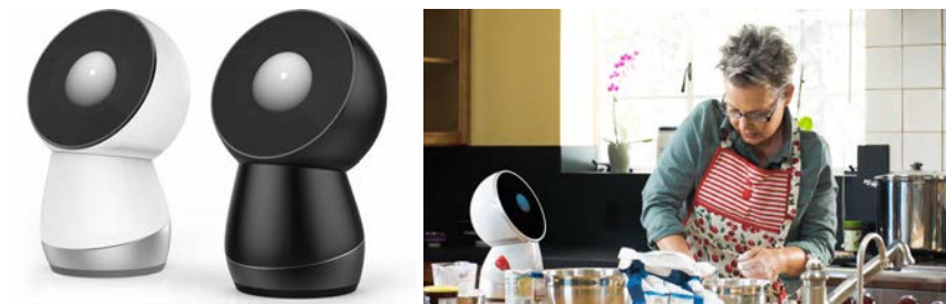
Figure 2.15: The social robot "Jibo". A user case is visible on the right, where Jibo is helping a user with her hands busy thanks to speech recognition. Images from http://www.myjibo.com/ .
