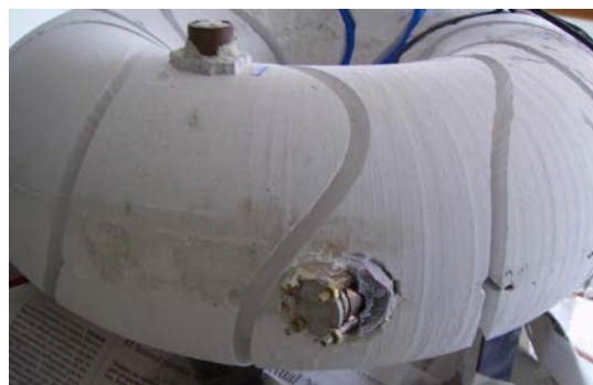
Fig. 2.8. Monolithic frame and grooves for the coils.
