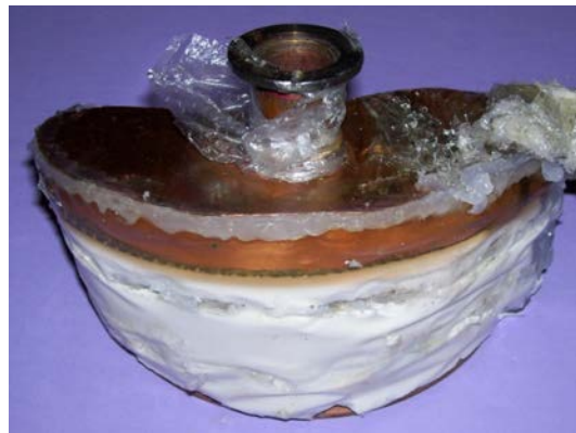
Fig. 6.15. Test of the liner vacuum vessel.
