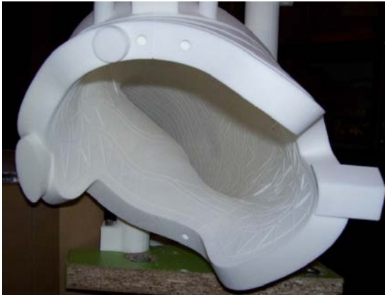
Fig. 7.5. Profile view of the frame structure. Three attachments for the large planar coil are visible.
