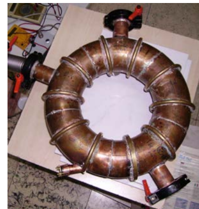
Fig. 2.5. UST_1 vacuum vessel.
