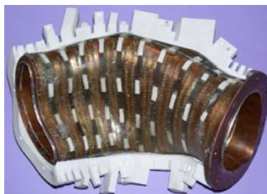
Fig. 7.44. Introduction of the VV in one half coil frame.
