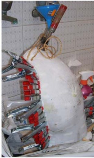
Fig. 7.19. Casting epoxy resin in the 3D printed nylon mould.
