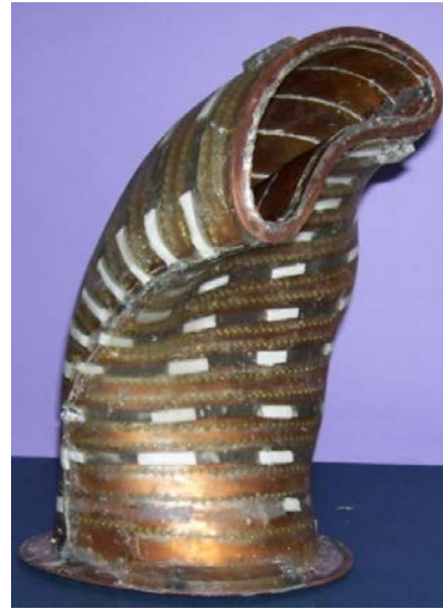
Fig. 7.20. Finished curved vacuum vessel sector.
