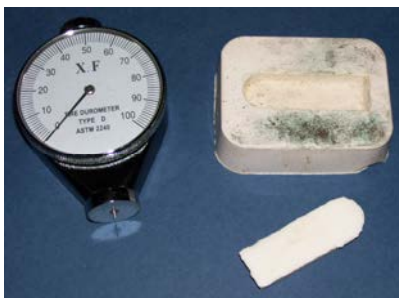
Fig. 6.2. Shore D hardness gauge, mould for specimen production and specimen.
