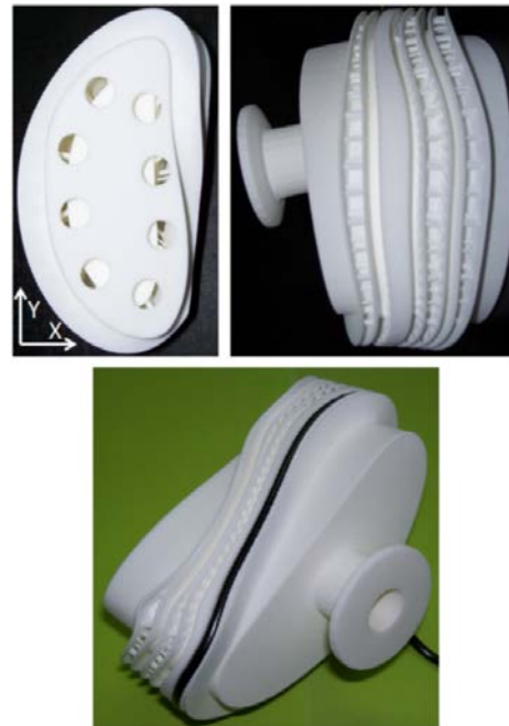
Fig. 6.9. Three views of the 3D printed mock-up coil frame. A vacuum flange type KF25, located at an abnormal position, was designed.
