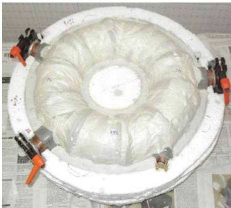
Fig. 2.6. Expanded polystyrene mould and vacuum vessel covered by a separation layer.
