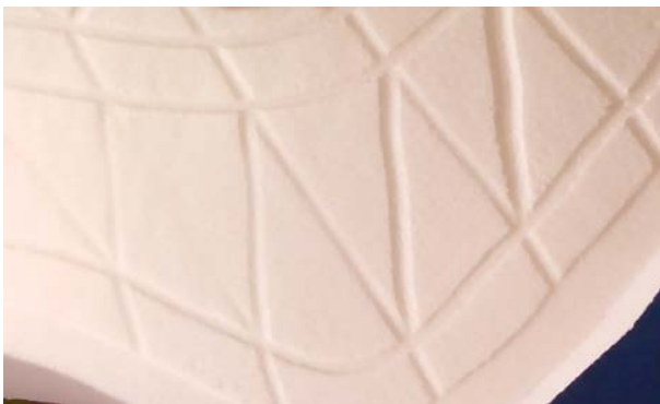
Fig. 7.7. Detail of the 3D printed reinforcement bars.
