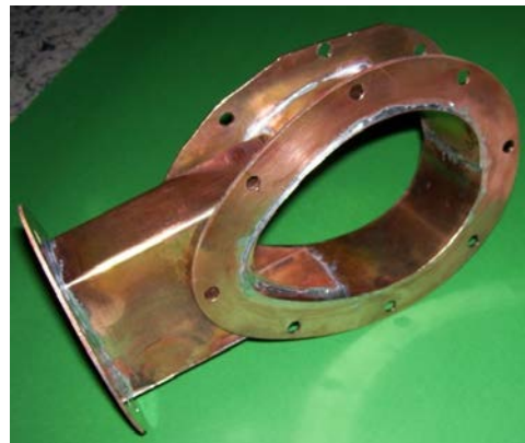
Fig. 7.22. Central vacuum vessel section.
