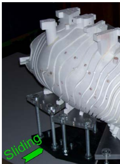
Fig. 7.41. Flat smooth base and sliding tables on the base.
