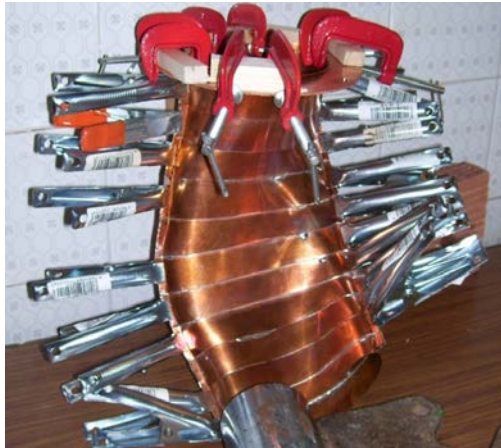
Fig. 7.15. Fixations to solder the large flange on the joined halves.
