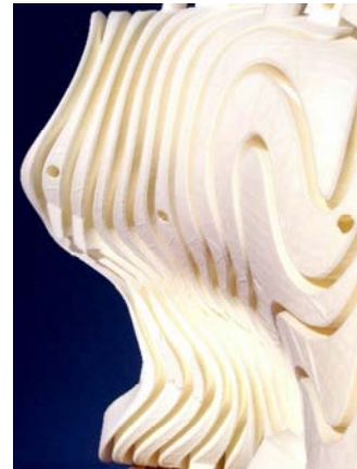
Fig. 7.8. Detail of a section of very contorted modular coils. Holes for the extraction of internal nylon powder are also visible.
