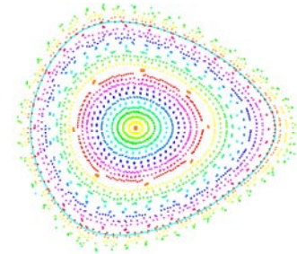
Fig. 3.5. Poincaré plot at \varphi=0 for LCFS' resulting from 180 coils. LCFS' is the solid cyan line.
