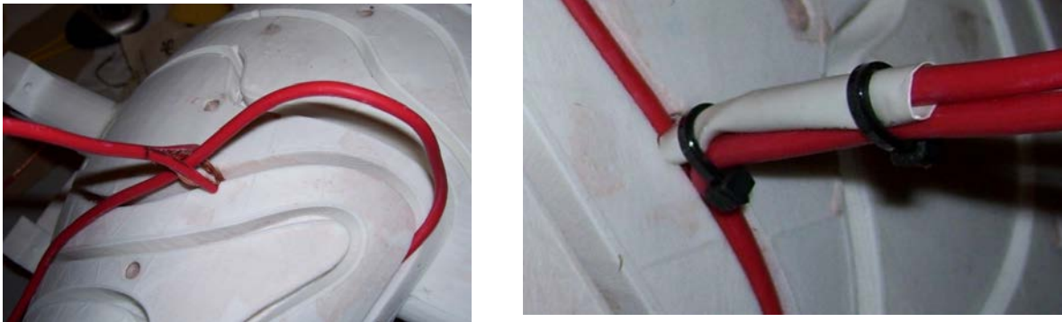
Fig. 7.26. Winding process through the opening between copper filament bunches (left). Finalised winding of three turns. The heat shrink sleeve was not heated yet in this picture, (right).
