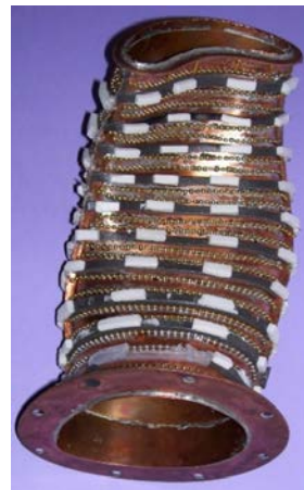
Fig. 7.18. Finished liner prepared for external resin casting. Shelf-gluing foam strips are located on solder lines.
