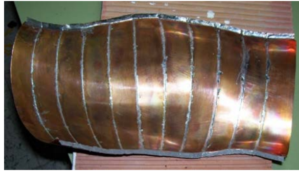
Fig. 7.14. Finished half vacuum vessel sector. It is pretinned at the lateral ribs with Bi-Sn solder.
