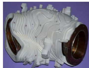
Fig. 7.45. Closure with the second half coil frame.
