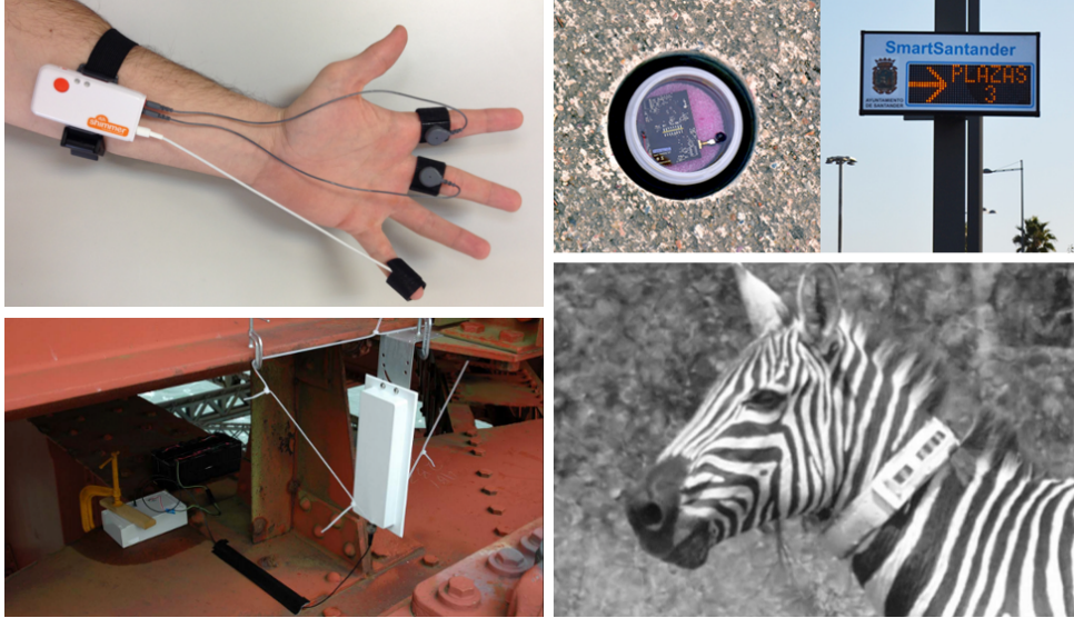
Figure 1.4: Example of applications of WSNs. Top left: Stress monitoring with Galvanic Skin Response (GSR) and Blood Volume Pressure (BVP) sensors. Top right: Smart Parking in Santander (Spain) taken from [18]. Bottom left: Structural monitoring of Golden Gate Bridge, San Francisco (USA) taken from [68]. Bottom right: ZebraNet animal tracking project taken from [137].
