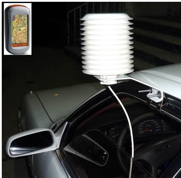
Figure 3-5 Mobile thermometer and Garmin Oregon 300 GPS device used during the mobile experiments.
