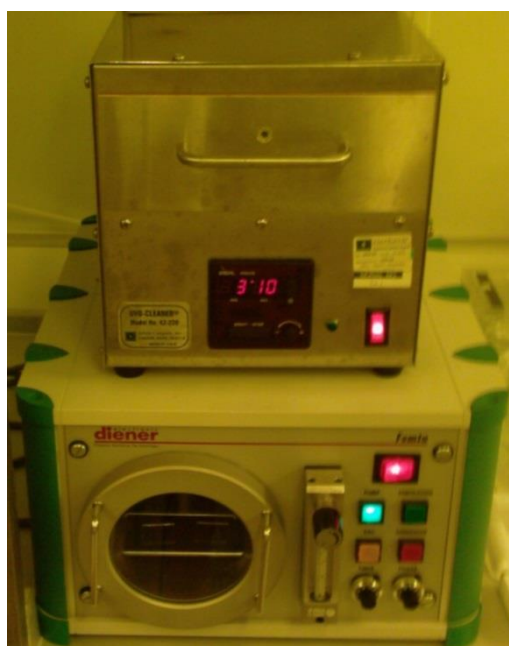
Figure 3.2: A Jelight UVO cleaner on top of a Electronic Diener Femto plasma cleaner, both were used to clean substrates.
