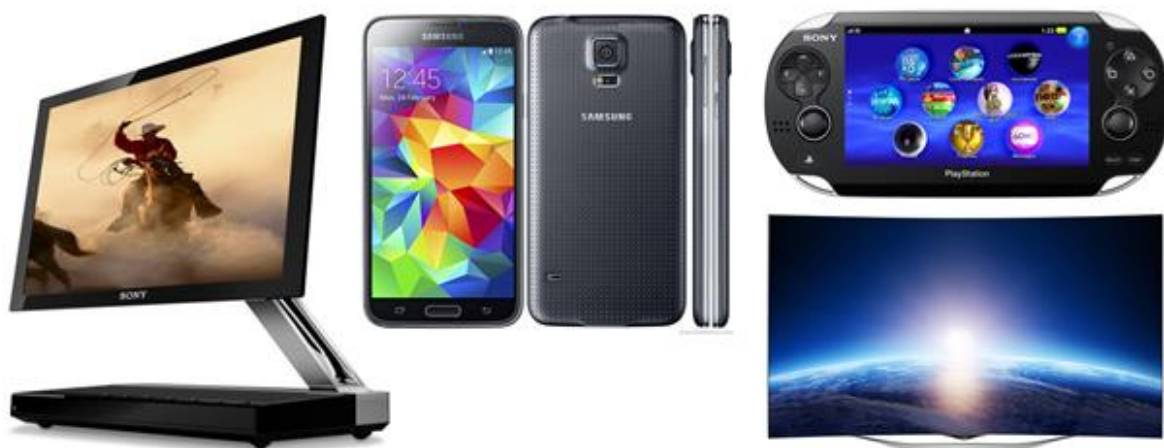
Figure 1.2: This figure shows the first OLED television made by Sony, the XEL-1, with a thickness of 3mm at its thinnest point. Also featured is the Samsung Galaxy S5, the Sony PlayStation Vita and the LG 55EC930V, all of which use OLED technology. [15-18]
