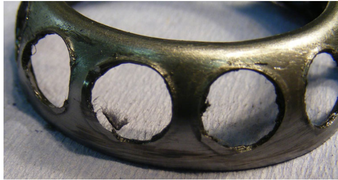
Figure 6.11: An example bearing cage suffering from degradation due to wear Stevens (2011)
