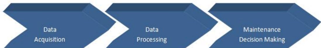
Figure 2.2: Condition based maintenance (CBM) process.
