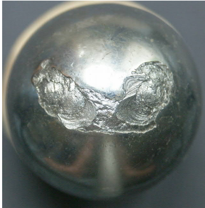
Figure 6.10: An example roller element (ball) suffering from surface fatigue Stevens (2011).
