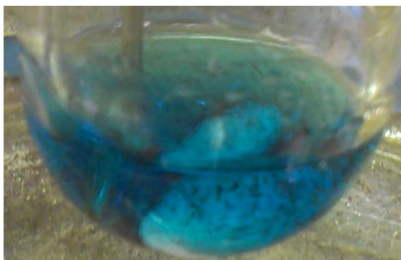
Figure 9: Pre-disproportionation of \text{CuBr} observed by the blue colour of the reaction mixture ( \text{CuBr}_2 ) and red-brown suspension of \text{Cu}(0)
