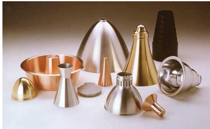
Figure 1.5: Smaller parts formed using the metal spinning process (Kleiner et al. (2005))
