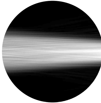
Figure 4.14 An x - z slice through the reconstructed field inside the sample. The grey scale shows the absolute value of the electric field inside.
