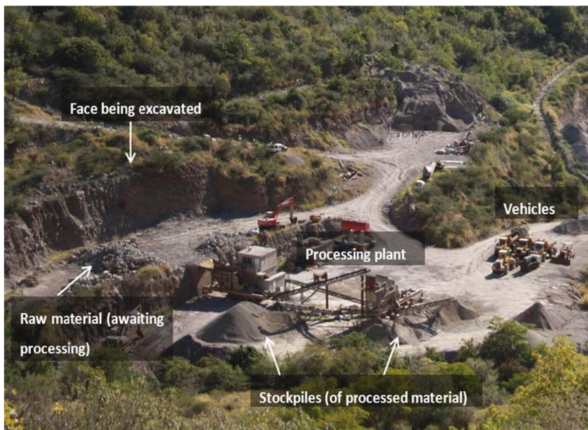
Figure 2.1 The typical components of a quarry (Phoenix quarry, Little Bay, Montserrat).
