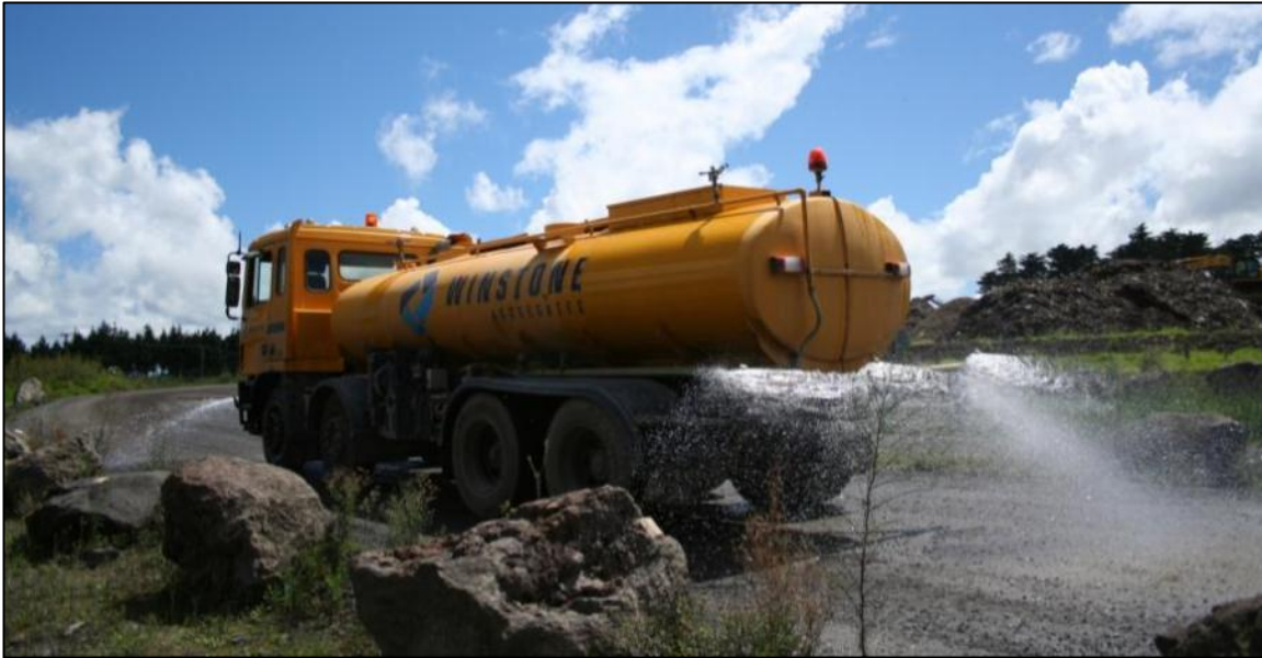
Figure 6.19 A water-cart spraying water to prevent the dust from the road from becoming re-suspended at Puketutu island quarry, New Zealand.
