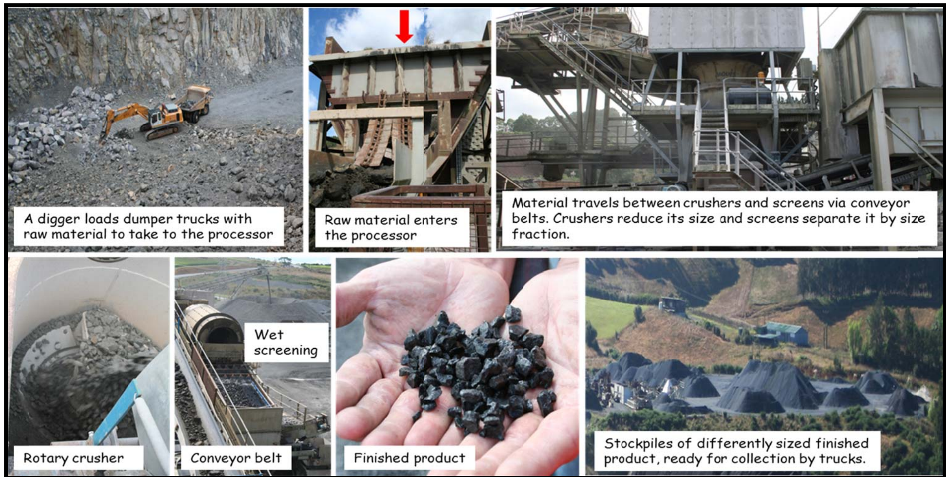
Figure 3.17 The processing of raw material into finished product. Quarry shown is Bombay quarry, South Auckland Volcanic Field, New Zealand.
