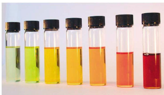
Figure 7: Solutions containing different sized CdSe quantum dots. 18
