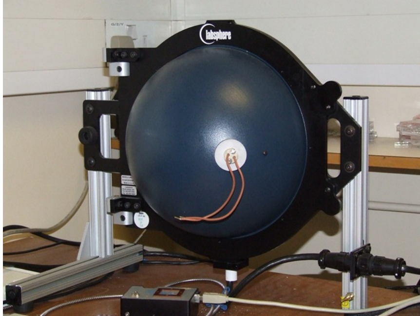
Figure 3.9: Photograph of the Labsphere LMS-100 10 inch integrating sphere used for device characterisation.
