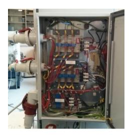
Figure 5-4 Voltage and Current Transducers
