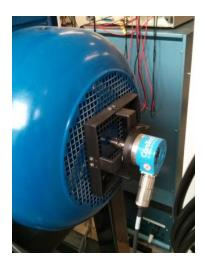
Figure 5-5 Encoder mounted on generator rotor shaft
