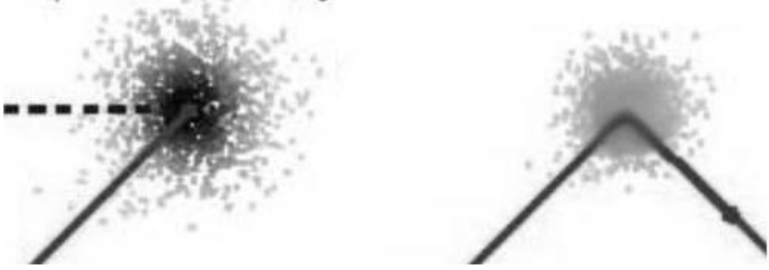
Figure 3.4: The result of resample step (Fox et al. 2000). A new set of particles is chosen so that each particle survives in proportion to its weight. The cloud of resampled particles is more condensed and smoother than un-resampled cloud.
