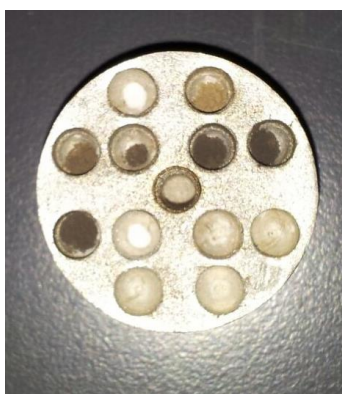
Figure 2.12: Oxygen fluorination line sample holder containing approx. 2mg of clay sample (brown) and standards (white) in the wells. Sample block approx. 3cm in diameter.
