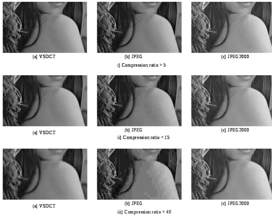
Figure 6: Zooming view of Lena test image at compression ratio of, i) 5, ii) 15 and iii) 40 encoded by (a) VSDCT image codec (b) JPEG, and (c) JPEG2000.
