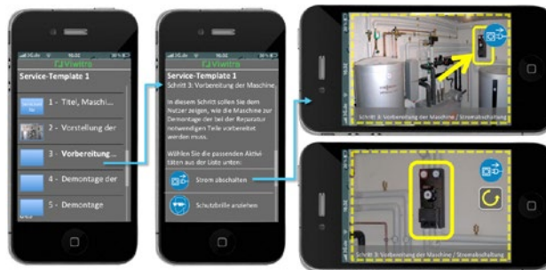
Fig. 12: Draft of the Template-guided filming and assembling of a service process with the suggested steps and content sequence
