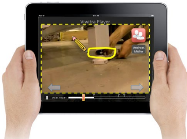
Fig. 10: Draft of the live video streaming based collaboration in which two employees observe the same video picture and can draw on it
