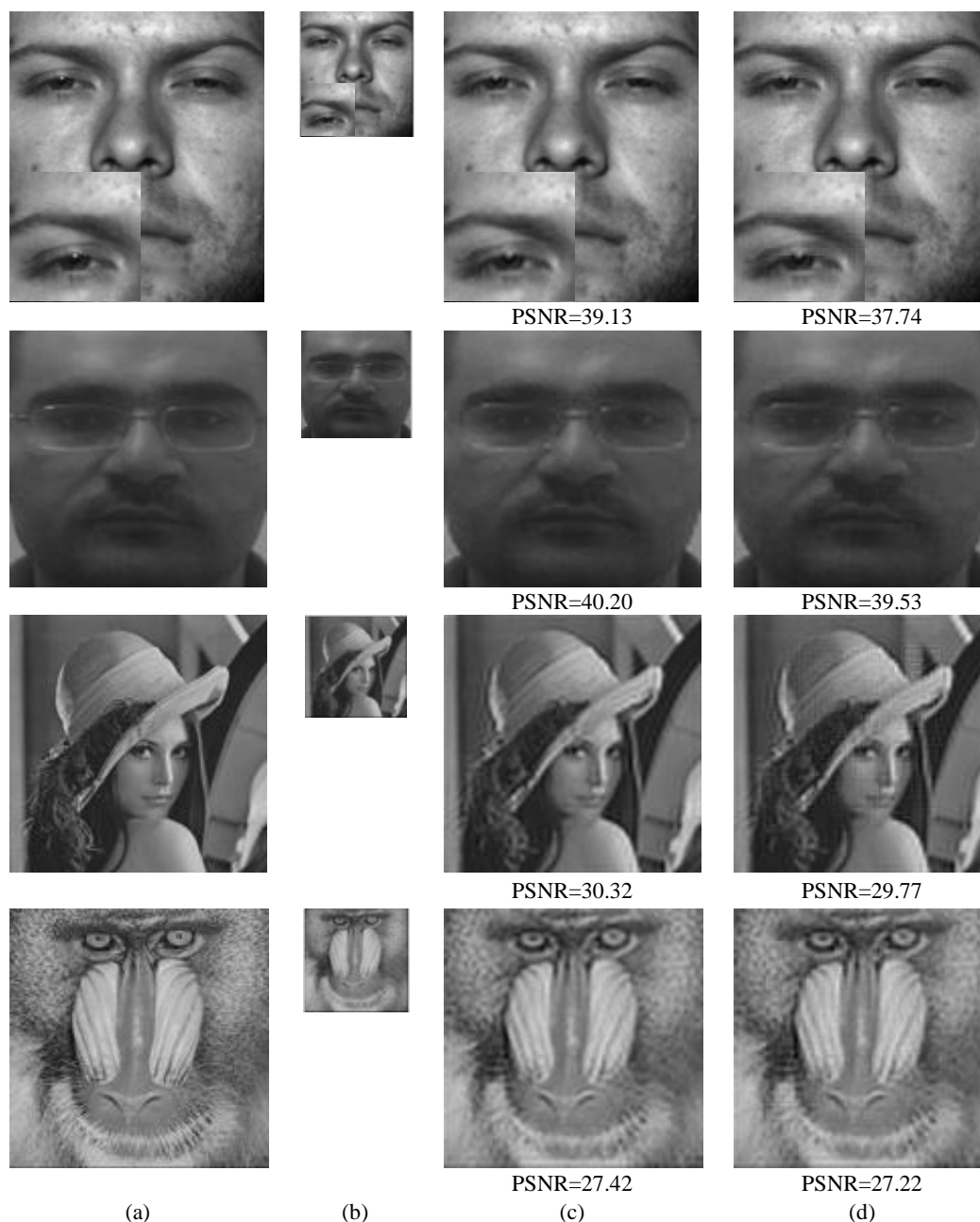
Figure 4.9: Comparisons of PSNR values between enhanced images, (a) First column: the original image. (b) Second column: the LR image generated by blurring and down sampling the original image. (c) Third column: super-resolved image by a factor of 2 using SR by LD-Sp method. (d) Fourth column: the super resolved image by a factor of 2 using SR by LD-WD method.
