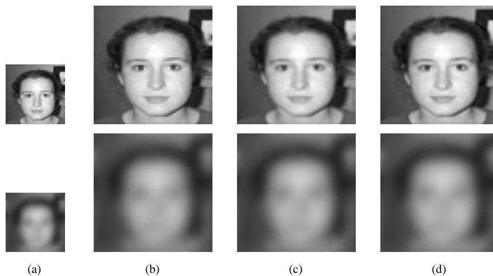
Figure 2.3: Well-known interpolation methods: the first column (a) original LR images with good and bad quality, the second column (b) nearest interpolation, the third column (c) bilinear interpolation, and the four column (d) bi-cubic interpolation.
