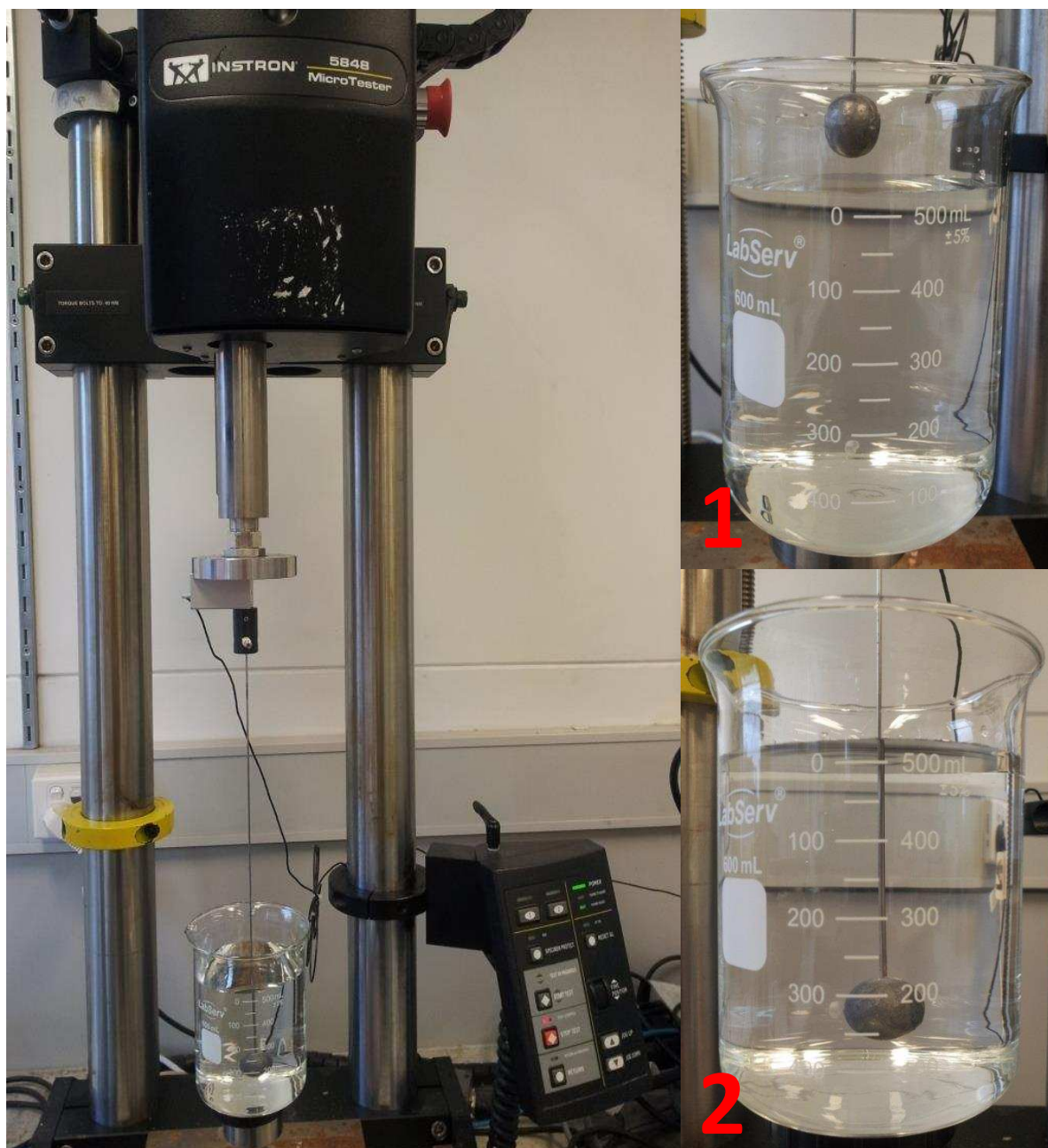
Figure 1 Creeping sphere test using Instron microtester; the force is measured during movement of the sphere from 1 to 2 (downward movement) and then 2 to 1 (upward movement). The medium is water in the photograph
