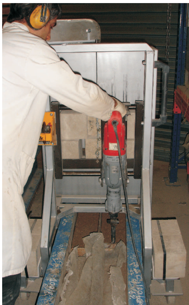
Figure 4. RCC compaction rig
