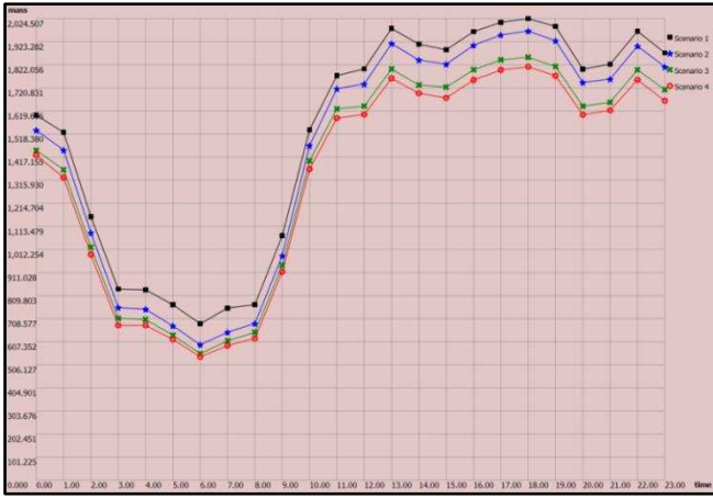
Figure 5: CO 2 emission (kg/h) of the network in Figure 3 as a function of time (h), under the five scenarios shown in Table 2. For clarity, the curve for Scenario 5 is not shown as it entirely overlaps that of Scenario 4.
