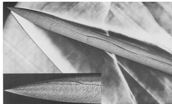
a) Experimental composite Schlieren/Oil flow photograph
