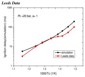
**Fig. 3** Comparison of predicted ignition delays with Leeds data for conditions of 20 bar under stoichiometric conditions of  $\phi = 1$
