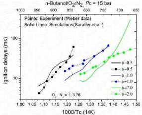
**Fig 1** Comparison of predicted ignition delays with experimental data from Weber et al. for conditions of 15 bar and = 0.5-2.0
