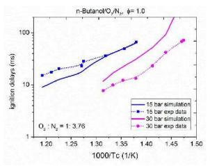
**Fig. 2** Comparison of predicted ignition delays with experimental data for = 1 at 15 bar and 30 bar
