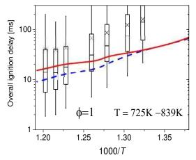
**Fig. 4** Comparison of predicted ignition delays (blue) with Weber data (red). Boxes - 25<sup>th</sup> and 75<sup>th</sup> percentiles; whiskers - 5th and 95<sup>th</sup> percentiles
