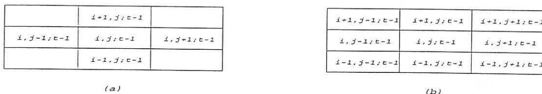
Figure 2: Examples of neighbourhoods for a two-dimensional CA (a) 5-site von Neumann neighbourhood (b) 9-site Moore neighbourhood
