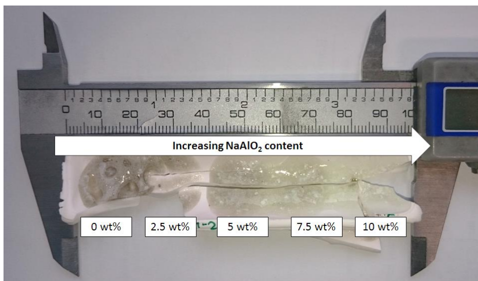
Figure 6.1 – Products formed by the heat treatment of 1g, 10mm diameter CSXC-CLINO pellets with the addition of NaAlO 2 between 0 wt % - 10 wt % at 1200 °C for 2 hours.
