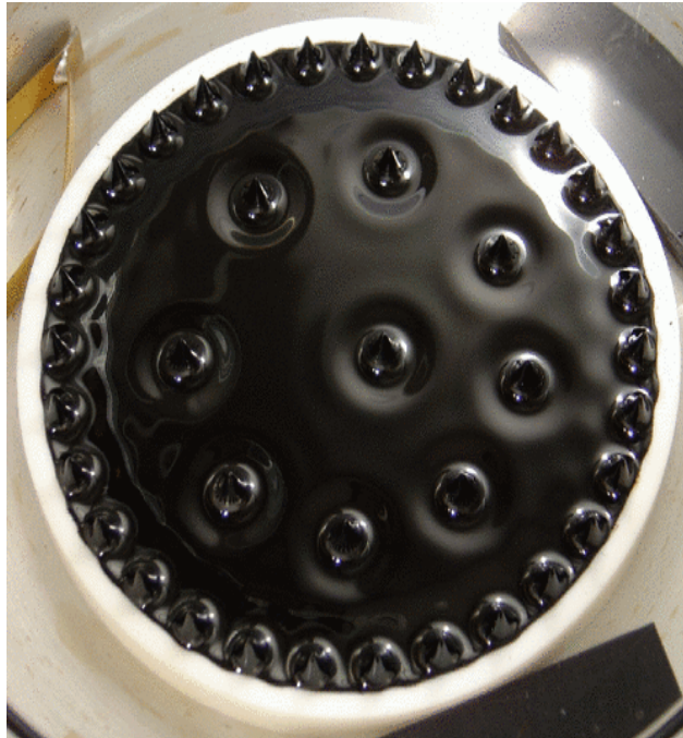
Figure 1.1: Soliton-like structure on the surface of a ferrofluid generated by applying magnetic field vertically. Figure is reprinted from [68], and the copyright (2005) is by the American Physical Society.
