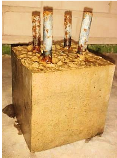
Figure 5.1.2 An example of the arrangement of four reinforced bars in CSA concrete
