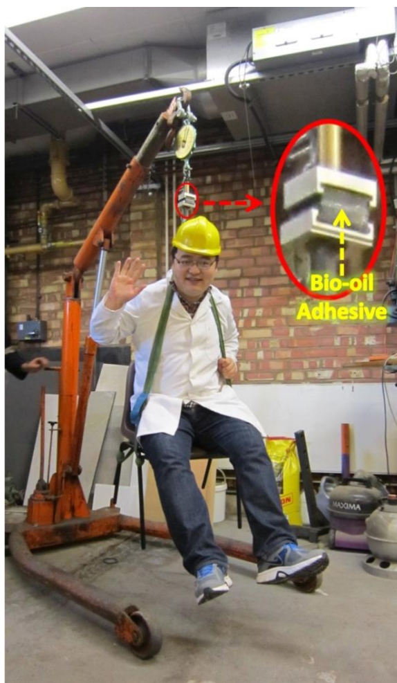
Figure 47: Adhesion strength test of the waste office paper derived organic phase bio-oil. The tested specimen is Al plates adhered by the crude, waste office paper derived organic phase bio-oil at 160 °C for 8 h curing. (Originally in colour)
