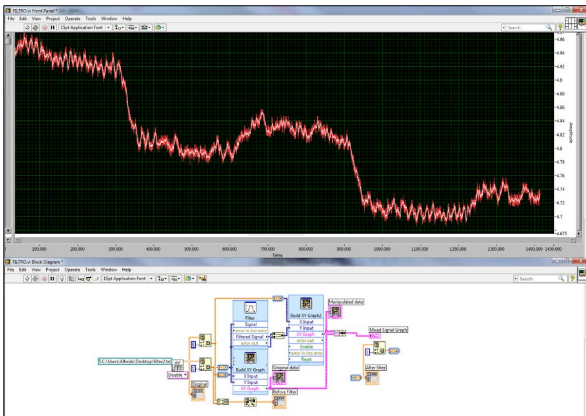
Figure 5.20: Front panel (top) and block diagram (bottom) of the filter designed in LabView. The front panel represents the signal before (red line) and after (white line) the signal treatment. The block diagram represents the programming code of the digital filter.
