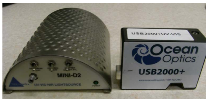
Figure 3.12: The spectroscopy apparatus. Left: Light source, right: spectrometer.
