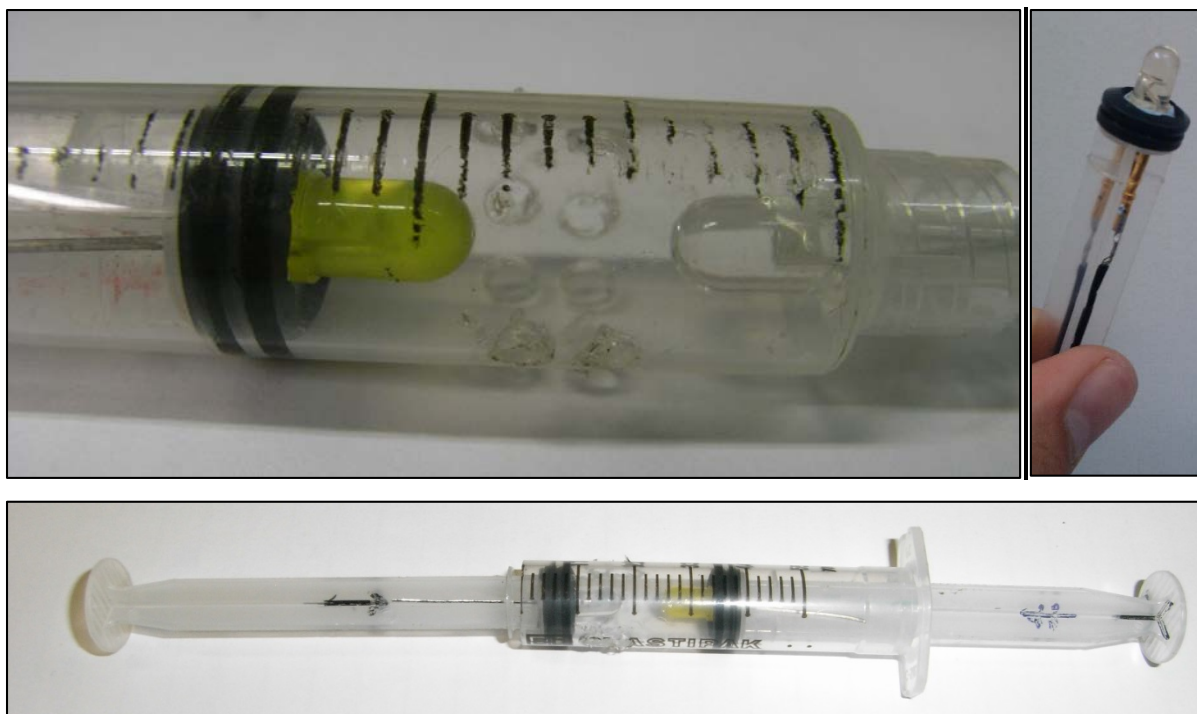
Figure 5.11: Photos of the syringe proto-type, which allowed easy variation of the LED-receiver distance.
