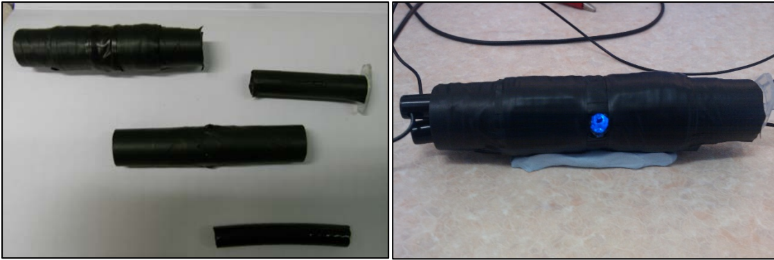
Figure 5.7: Left: Different light isolators that kept the sensing pair away from undesired sources of illumination. Right: operating prototype of a Phototransistor-LED pair.
