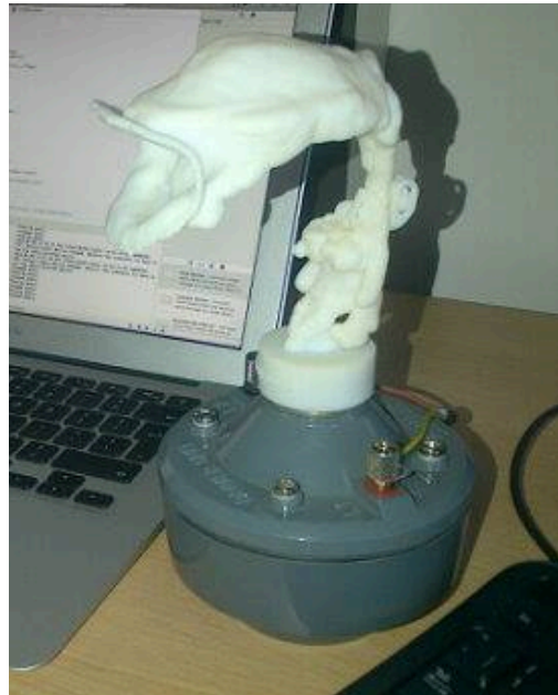
Figure 3.10 – A 3D printed vocal tract model for a sung /A/ vowel. The loudspeaker is attached via a seal at the glottis end.
