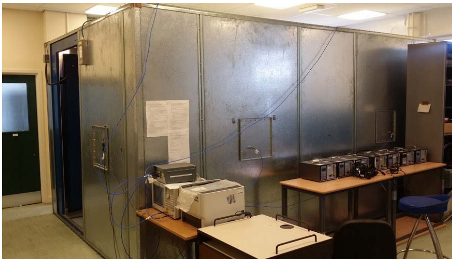
Figure 1. Resonant cavity perturbation equipment: screened room, network analyser, switching unit and RF cables
