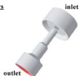
Figure 4. Presentation of the high-pressure nozzle disintegrator. (Reproduced with permission from Bałdyga et al. [44]).
