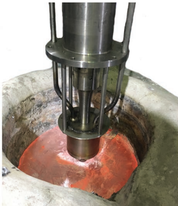
Fig. 1. Ultrasonic treatment of molten aluminium
