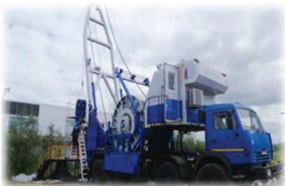
Fig. 7. Photograph of the wireline truck for sonochemical treatment of horizontal wells in working position
