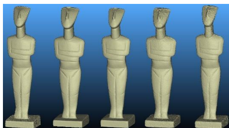
Figure 6: Agisoft Metashape OBJ1 meshes (from left to right) P30, SL1 VIS, SL1 full, SL1 UVAb, SL1 IRA
