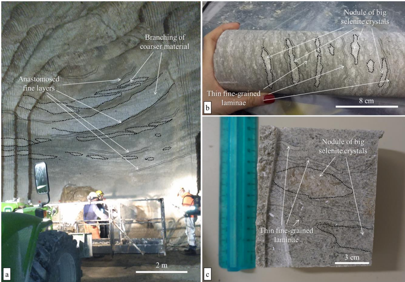
Figure 1 a. Excavation face in a gypsum underground quarry in Monferrato (NW Italy). It is evident the typical structure of the branching selenite gypsum, with branches of coarse material surrounded by anastomosed fine layers. b. Core sample of microcrystalline branching selenite gypsum, with nodules of big gypsum crystals surrounded by thin fine-grained laminae. c. Hand sample, with a more detailed scale, with nodules of big gypsum crystals surrounded by thin fine-grained laminae
