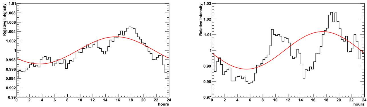
**Figure 4.** Sidereal time variations of the number of counts obtained in the  $10^{5.6} < N_{\text{ch}} < 10^{6.4}$  (left panel) and  $N_{\text{ch}} > 6.4$  (right panel) shower size intervals by applying the east–west method ( $\Delta t = 20$  minutes). The line represent the fitted first harmonic; amplitudes and phases are reported in Table 2.
