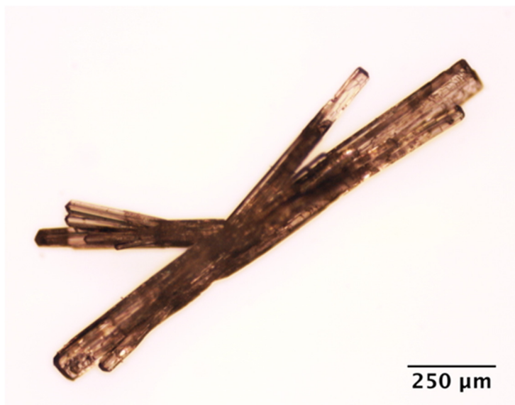
Figure 12 – Optical micrograph of \text{Ce}_2(\text{NDC})_3(\text{DMF})_2 crystals.
