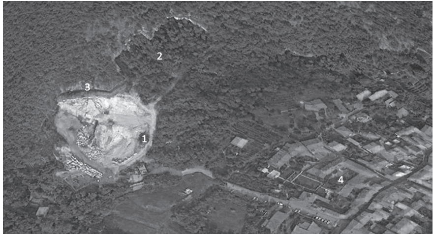
Fig 1. Aerial view of the white and pink Zandobbio marble quarry: 1) active quarry, 2) old quarry, 3) top face treated to accelerate aging, 4) Zandobbio village. didascalìa in italiano
