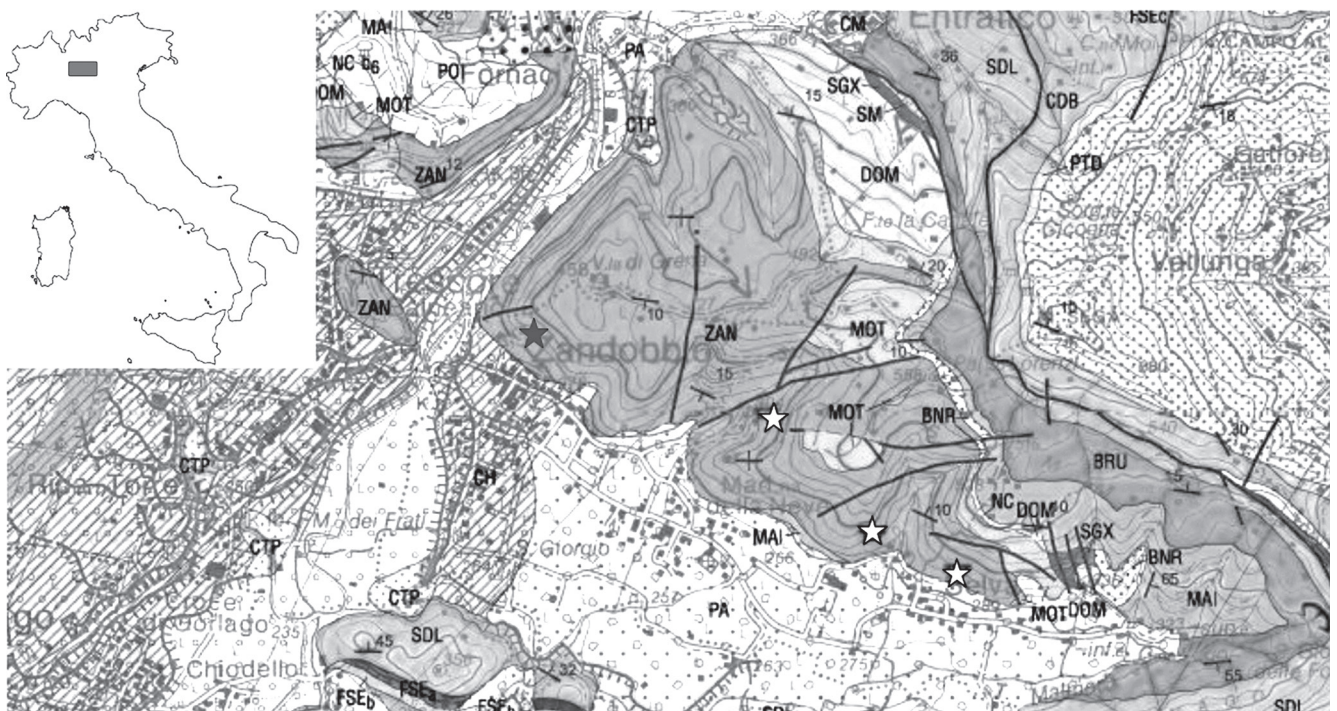
Fig. 3. Geological map of the Zandobbio Marble area, modified from “Carta Geologica d'Italia (1:50.000)” with overprinted quarries (blue star: ornamental stone quarry; white stars: quarries for industrial material). Legend: PA: massive or roughly stratified silt and silty clay, slope or debris flow deposit; CTP: roughly stratified conglomerate with arenaceous matrix; CH: gravel with subrounded clasts (alluvial deposits); clayey-silty diamicton (debris flow deposits); PTD: alternance of sandstones and shales; CDB: Grey silty marlstones; FSE: red marlstones, chaotic calcareous bodies, thin bedded turbiditic sandstones; SDL: grey marlstone and calcareous marlstone, locally reddish; BRU: black to purple red shales and marlstones followed by thick alternances of arenaceous-pelitic and marly calcareous turbidites; MAI: succession of white, light grey or cream coloured calcilitites; BNR: paraconglomerate and limestone breccias; DOM: light grey, marly, chert-bearing limestones; ZAN (Zandobbio dolomite): dolomicrites and oolitic doloarenites, white or pink.
