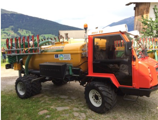
Fig. 3.1: the self-propelled high-precision digestate spreader (a) and the low-emission spreading system
