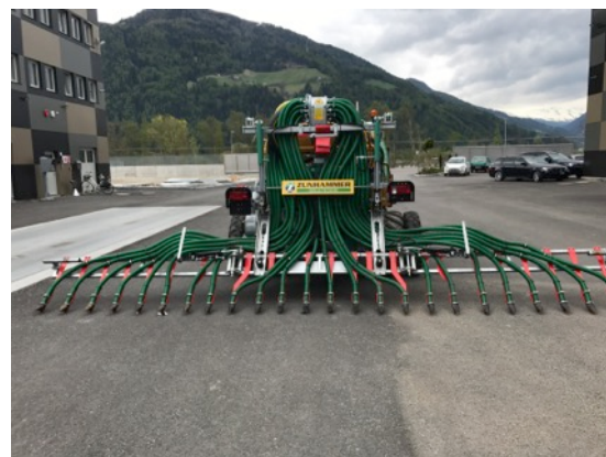
Fig. 3.1: the self-propelled high-precision digestate spreader (a) and the low-emission spreading system
