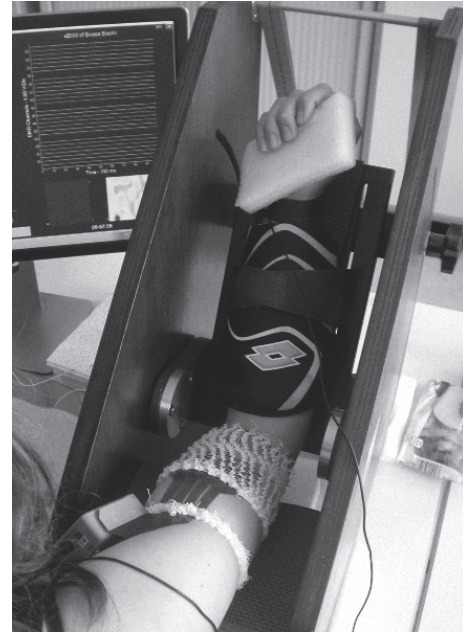
FIGURE 1: Electrode array position on biceps brachii muscle.
