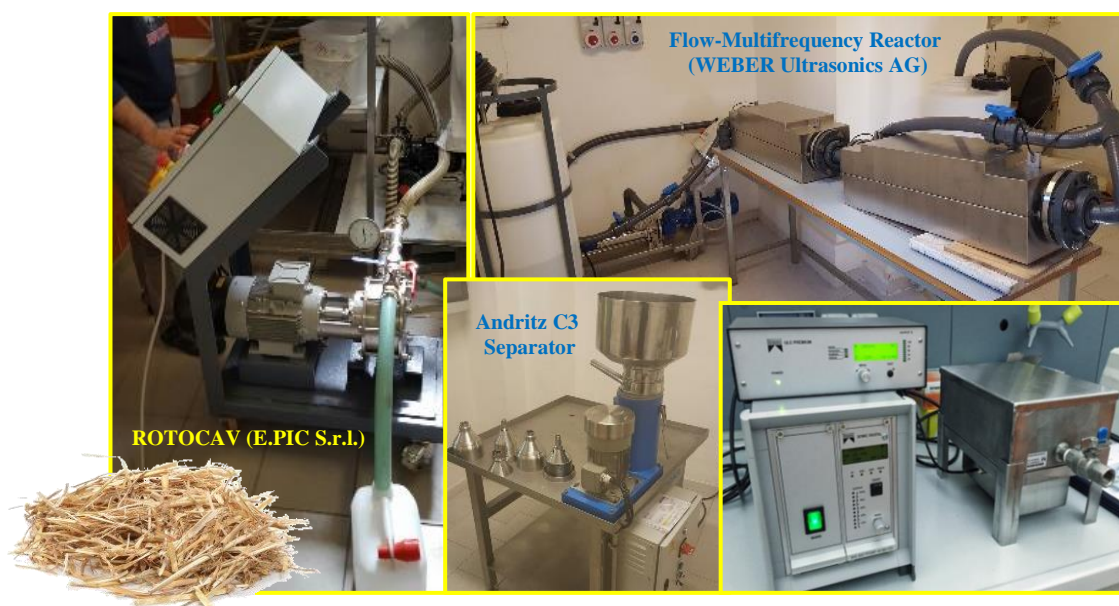
Figure 1. HC (left) and high-intensity US reactors (right) for wheat straw pre-treatment.
