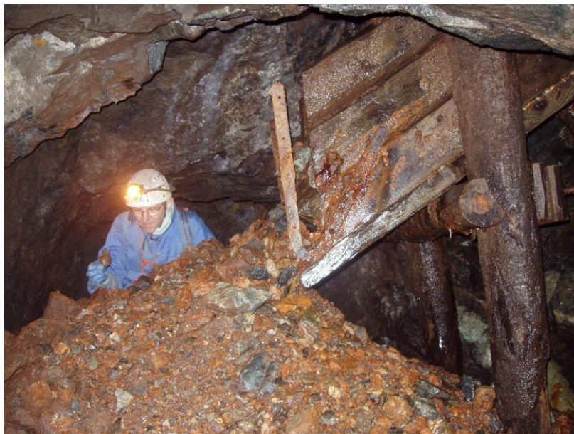
Figure 21. An original wood hopper, still presenting the original exploited mineral
