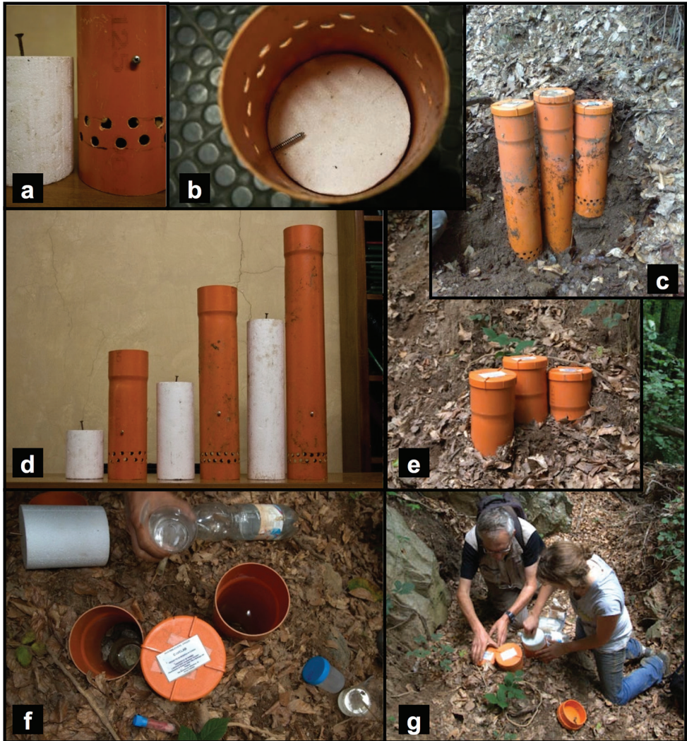
Figure 3. a sampling holes (details) b Blocking screw c installation of an MSS-triplet d SSD of three different length e MSS-triplet buried in the ground f, g renewing the pitfall trap inside the SSD. Photo credits: Elena Piano.
