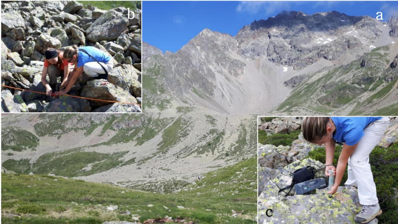
Figure 2 - The Paradisin rock glacier (a), on the Swiss side of the Val Viola (Poschiavo Valley) that has been investigated by means of electrical resistivity tomography (ERT) (b) and Schmidt hammer (c) methods.
