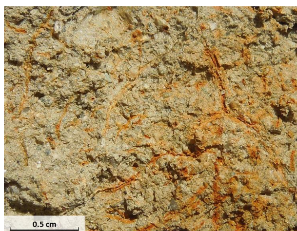
Figure 1. Exposed surface after breaking the soil, showing several oxidised root channels within the reduced soil matrix.
